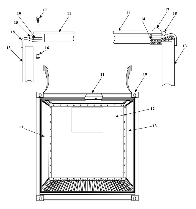
Figure 1. Roof Panel Removal (Sheet 2 of 2)
