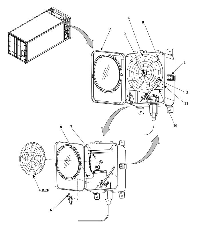
Figure 2. Temperature Recorder
