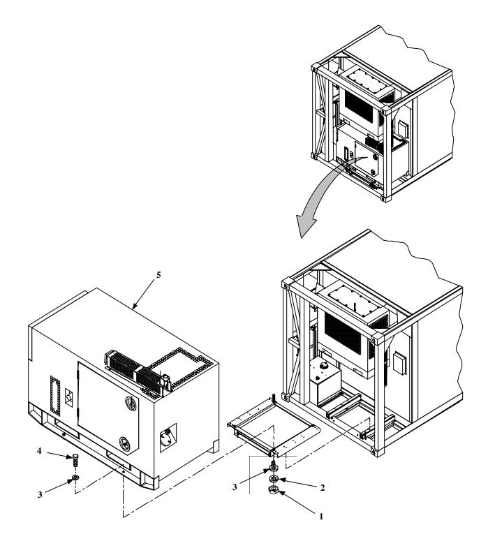
Figure 2. Generator Set and Mounting Hardware
