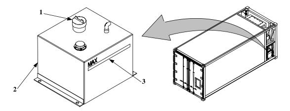
Figure 1. Generator Set Fuel Tank
