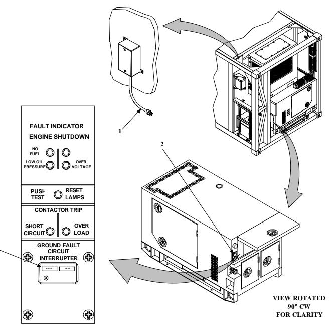
Figure 5. Light Cable and Ground Fault Interrupt Circuit Breaker
