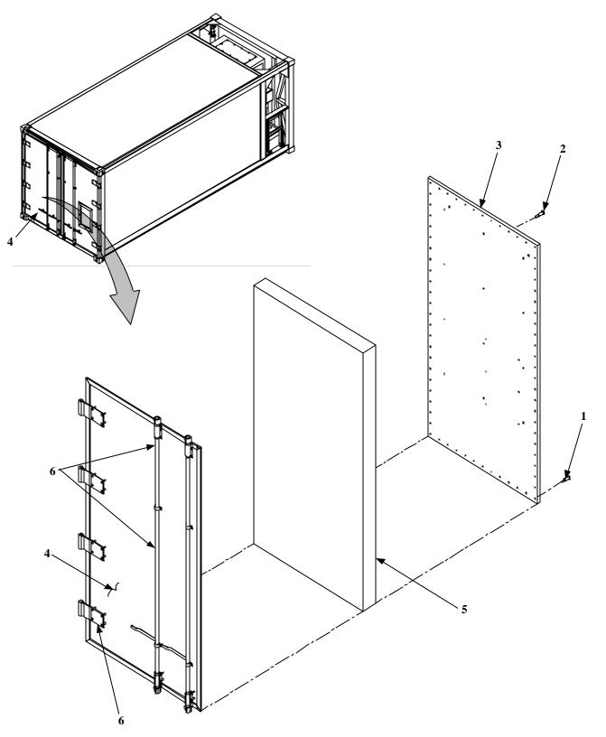
Figure 1. Rear Door, Left – Disassembly (Sheet 1 of 3)
