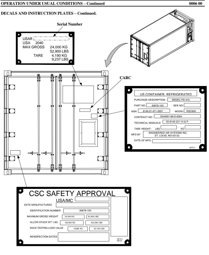
Figure 18. Container External View (Rear)
