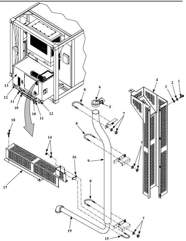
Figure 1. Exhaust Pipe Assemblies
