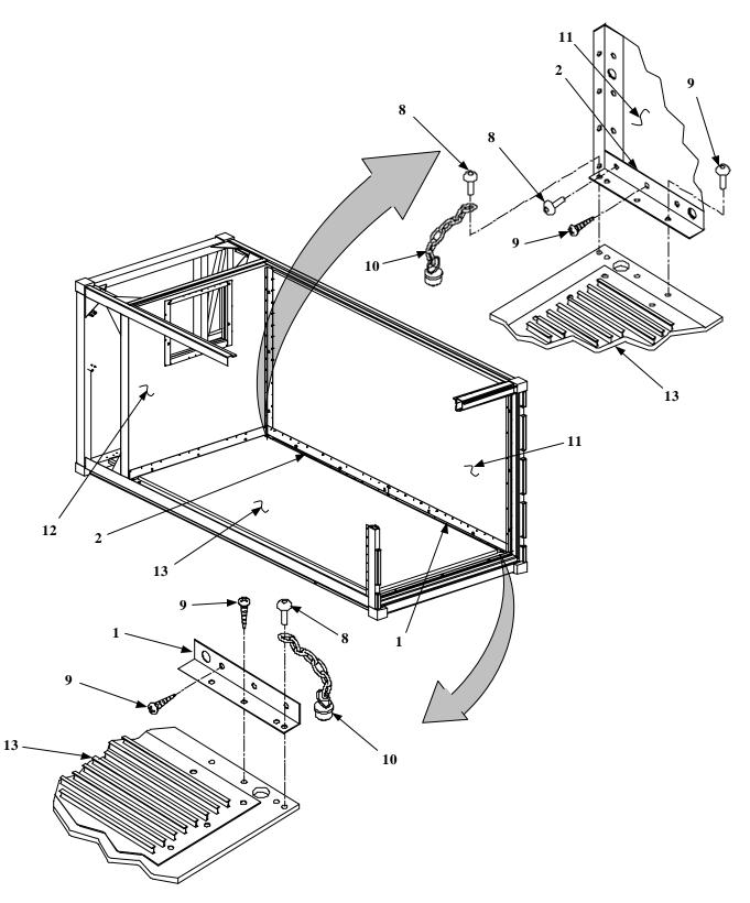
Figure 1. Panel Removal (Sheet 2 of 4)
