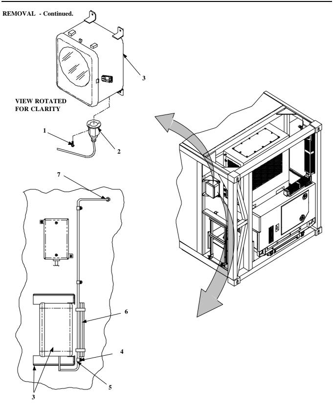
Figure 1. Recording Thermometer Element, Removal (Sheet 1 of 2)
