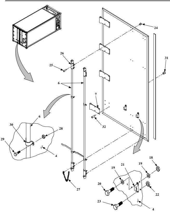
Figure 1. Rear Door, Left – Disassembly (Sheet 3 of 3)
