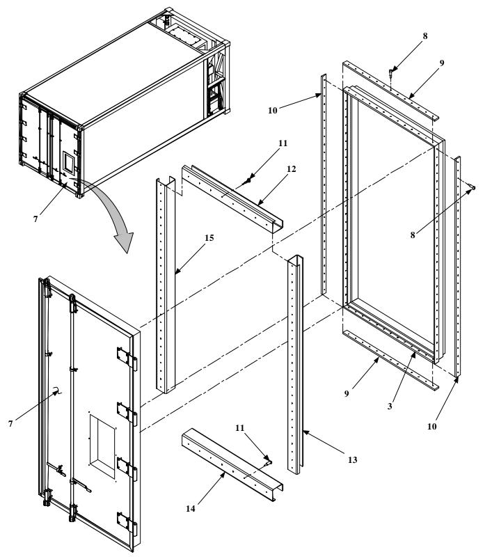
Figure 1. Disassembly (Sheet 2 of 3)
