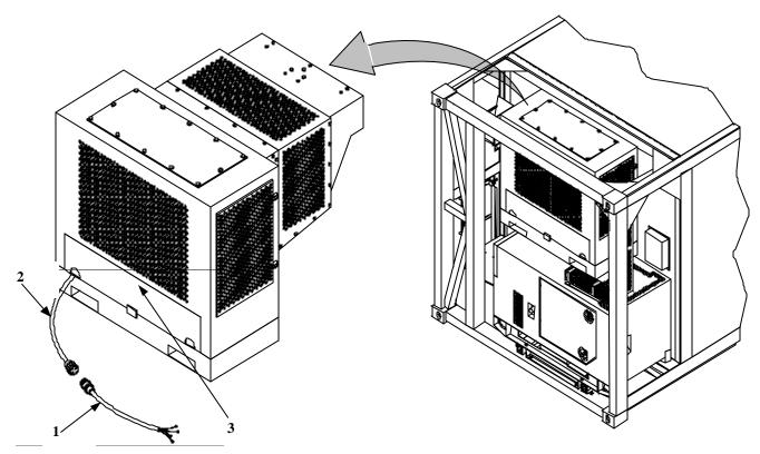
Figure 4. Air Conditioner Input Power Cable
