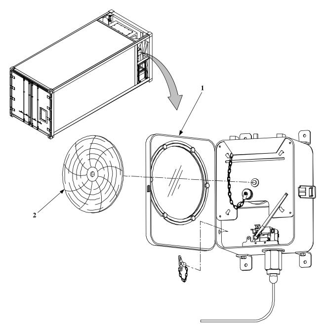
**Figure 2. Temperature Recorder**
