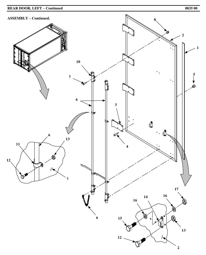
Figure 2. Rear Door, Left – Assembly (Sheet 1 of 3)
