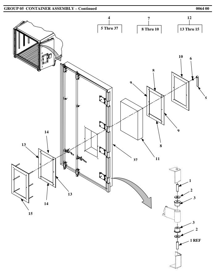
Figure 15. Right Hand Door Assembly (Sheet 1 of 4)
