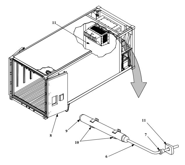
Figure 1. Recording Thermometer Element, Removal (Sheet 2 of 2)
