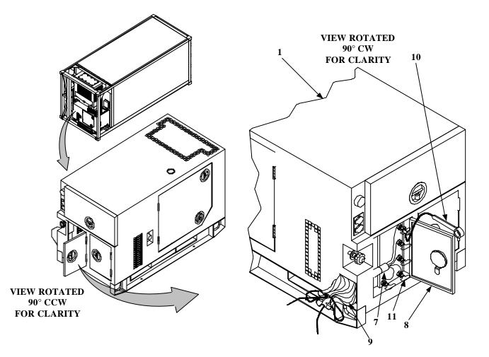
Figure 3. Generator Set Installation (Sheet 2 of 4)
