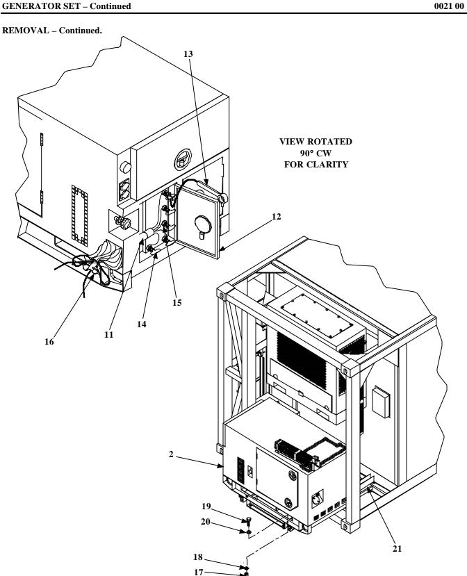
Figure 1. Generator Set Removal / Installation (Sheet 2 of 2)
