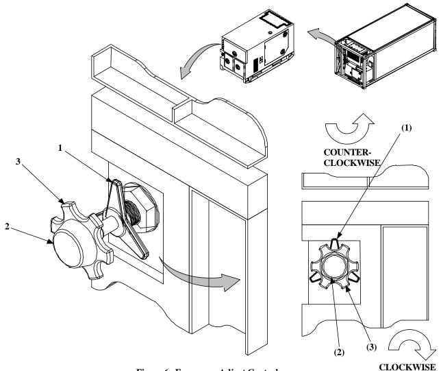
Figure 6. Frequency Adjust Control
