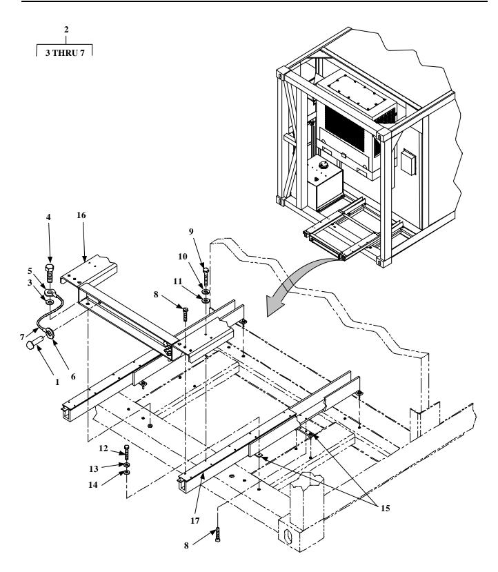
Figure 3. Generator Set Slide Unit and Mounting Hardware
