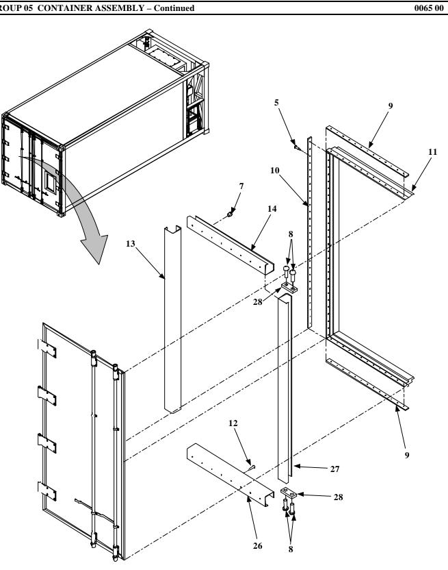
Figure 16. Left Hand Door Assembly (Sheet 2 of 3)
