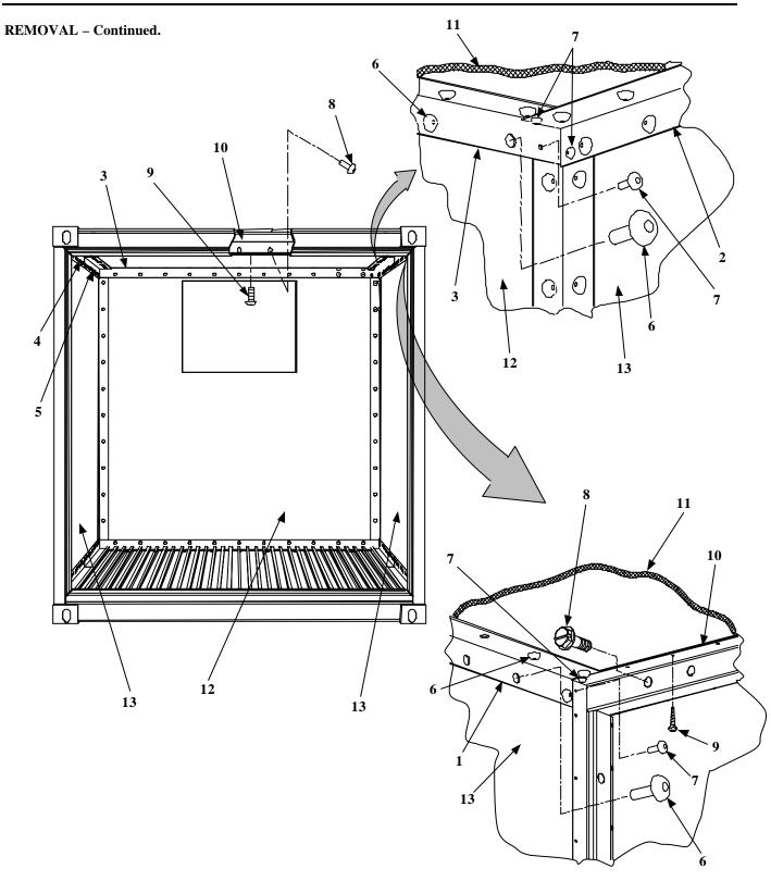
Figure 1. Roof Panel Removal (Sheet 1 of 2)
