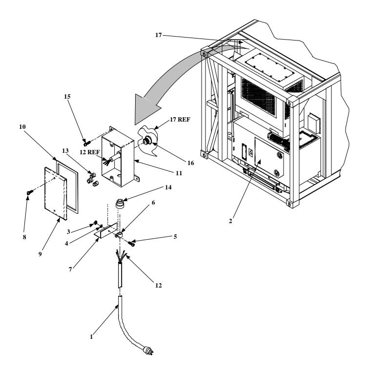
Figure 1. Light Assembly, Exterior
