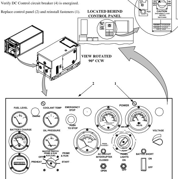
**Figure 2. Generator Set Preparation**
