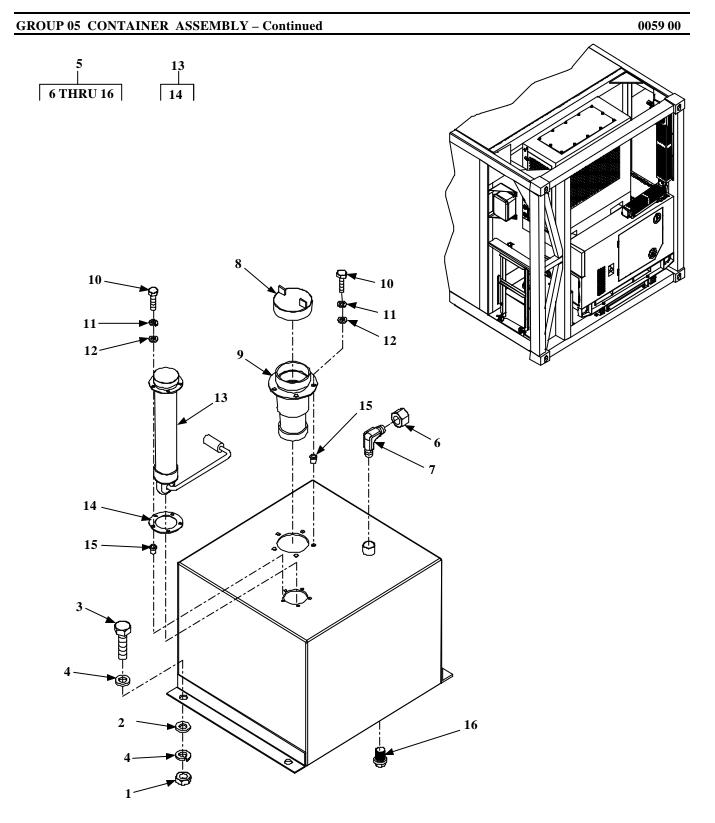
Figure 10. Fuel Tank Assembly and Mounting Hardware
