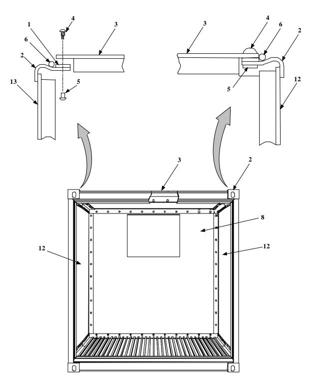
Figure 2. Roof Panel Installation (Sheet 1 of 2)
