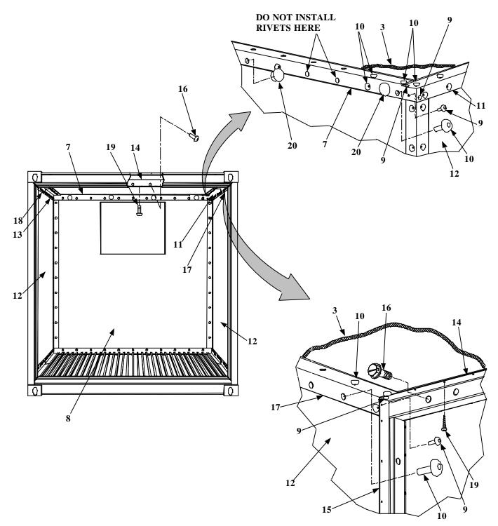
Figure 2. Roof Panel Installation (Sheet 2 of 2)
