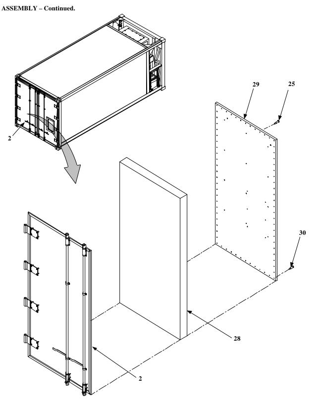
Figure 2. Rear Door, Left – Assembly (Sheet 3 of 3)
