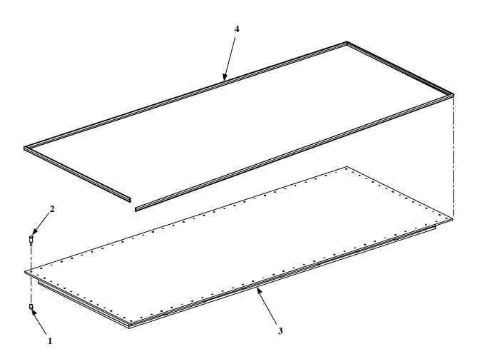
Figure 18. Roof Assembly
