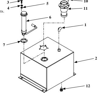
Figure 2. Fuel Tank Disassembly
