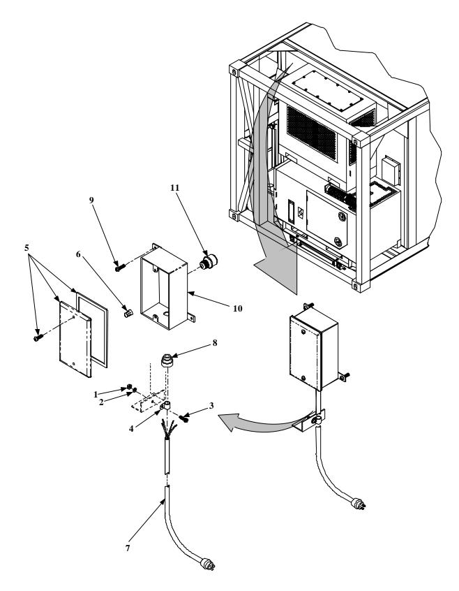
Figure 11. Power Cord and Connectors
