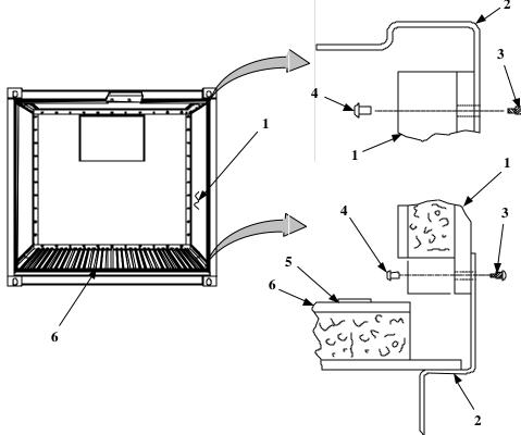
Figure 2. Panel Installation (Sheet 2 of 4)
