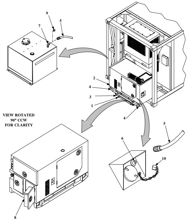
Figure 1. Generator Set Removal / Installation (Sheet 1 of 2)
