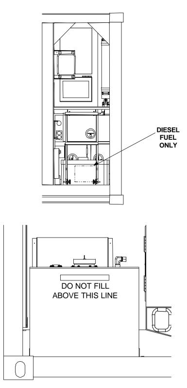
Figure 19. Container External View – Fuel Tank Markings
