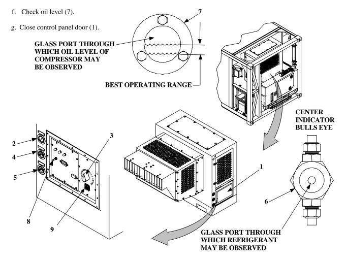
Figure 13. Refrigerated Container, Continuous Operation, Refrigeration Unit
