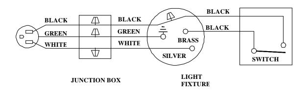
Figure 2. Wiring Schematic
