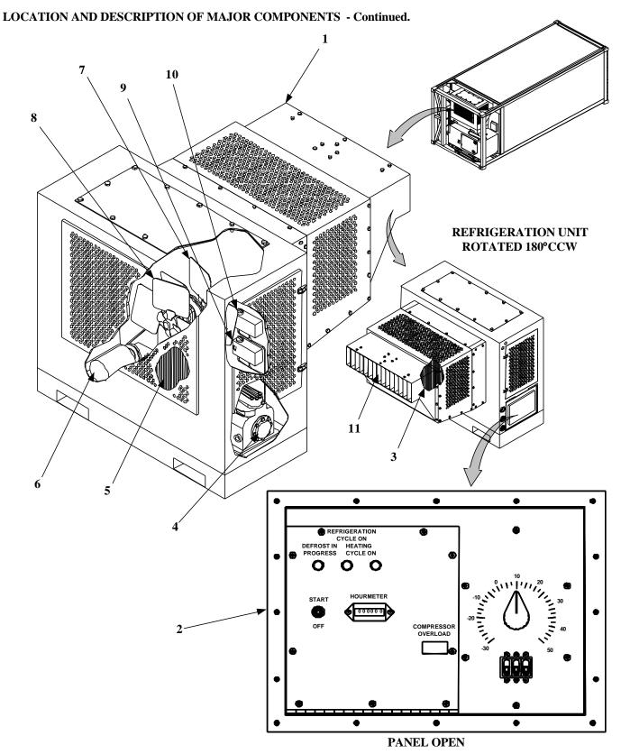
Figure 11. Refrigeration Unit Major Components 0002 00-15
