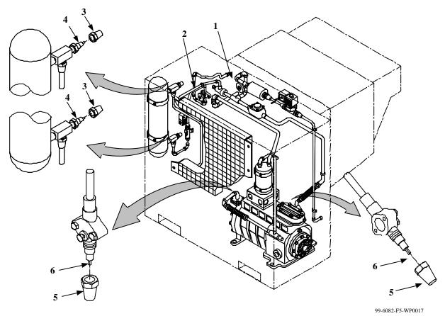
Figure 6. Refrigeration Valve Setting for Normal Operation
