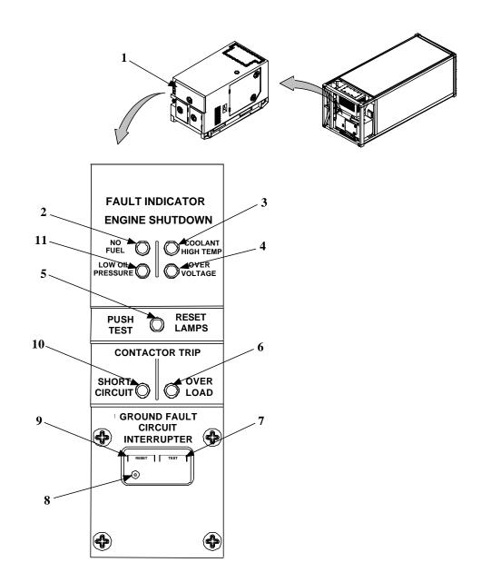
Figure 5. Malfunction Indicator Panel
