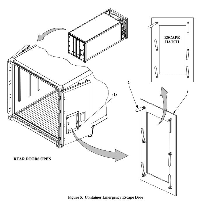
Escape Door (1, Figure 5). Provides emergency exit for personnel from inside refrigerated container.
