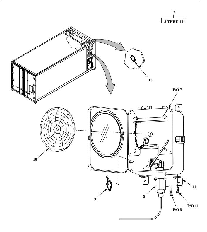
Figure 7. Temperature Recorder (Sheet 2 of 2)
