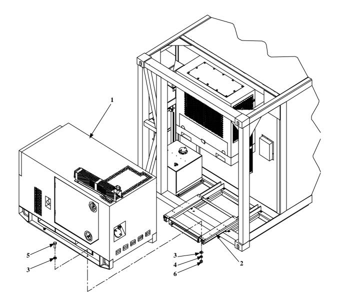
Figure 3. Generator Set Installation (Sheet 1 of 4)
