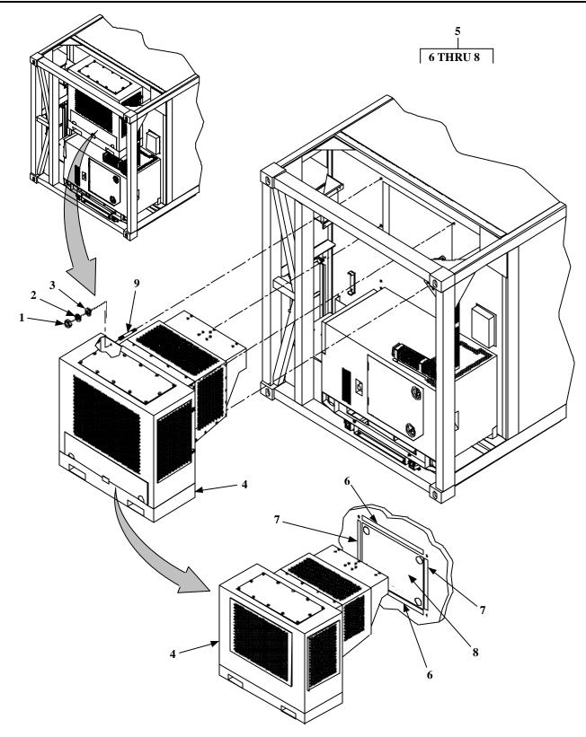
Figure 4. Refrigeration Unit and Mounting Hardware
