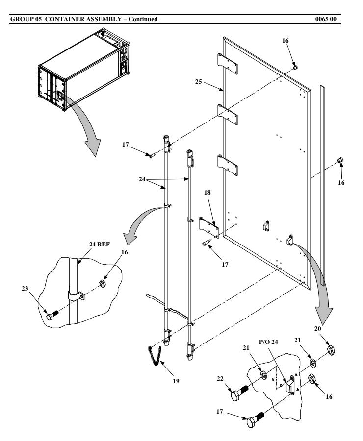
Figure 16. Left Hand Door Assembly (Sheet 3 of 3)
