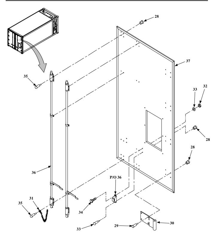
Figure 15. Right Hand Door Assembly (Sheet 4 of 4)
